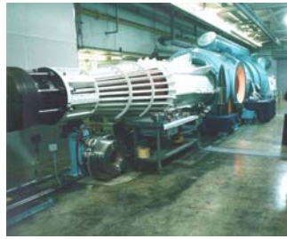
Wind Tunnel Internally And Vibrationally Isolated From Model And Optical Bench Component.
