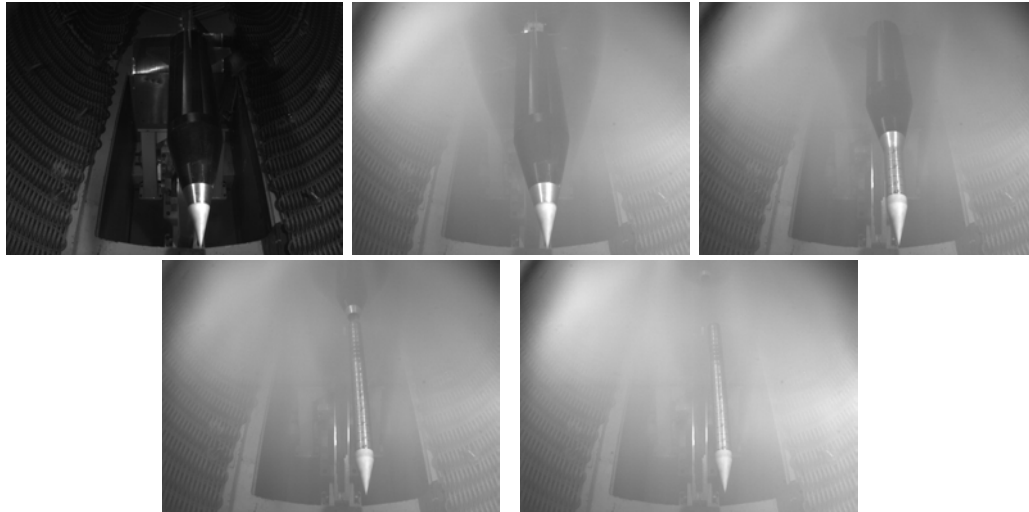
Figure 96: Sequence of High Speed Images taken during Penetrator/Booster Separation
