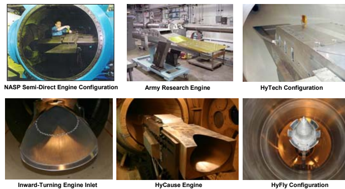
Figure 62: Scramjet Engines Tested in LENS Facility
